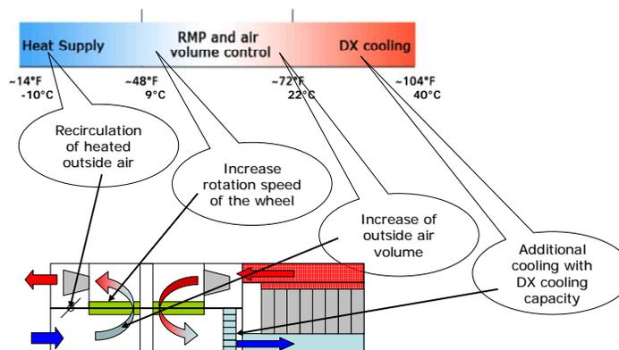
Figure 4. Illustration of the KyotoCooling control system.
