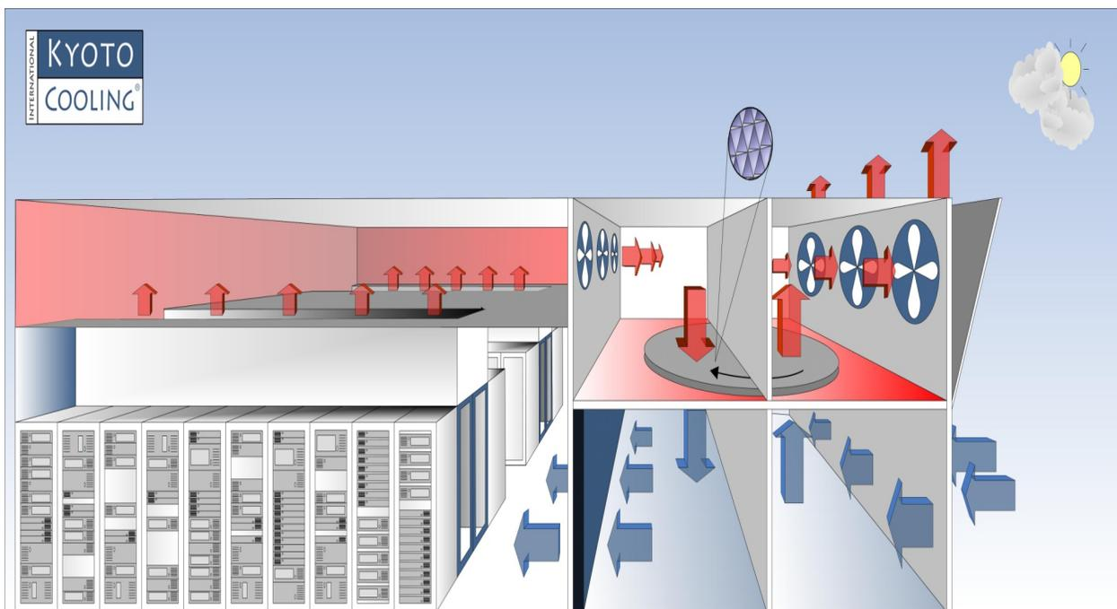
Figure 3. A general overview of the KyotoCooling installation and airflow patterns.
