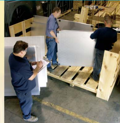
All SiteBilt components are inspected and staged to suit unit construction plans – then crated for on-site delivery.
