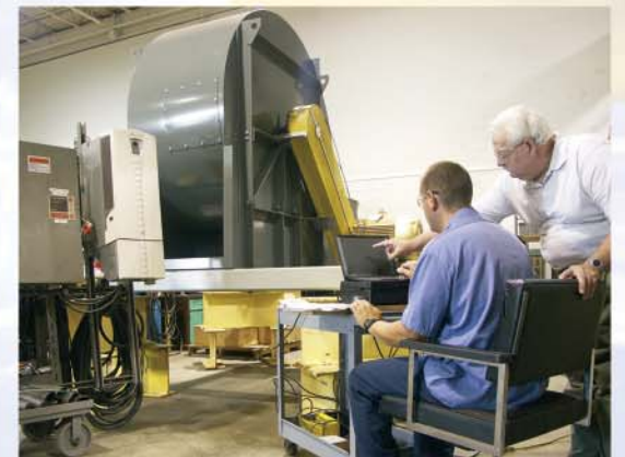
Critical components, such as fans, are dynamically balanced and tested at the factory.
